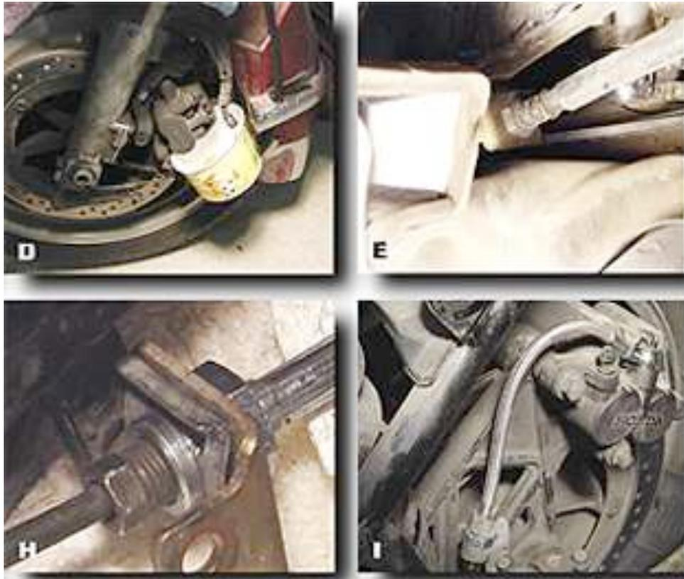
The next line is the one that connects the front left caliper to the rear master cylinder. Remove the right lower fairing panel. Remove the right cooling fan. Remove the right lower inner panel (the one the compressor controls are mounted in). Remove the right side panel that covers the battery. Remove the left front rotor cover.
