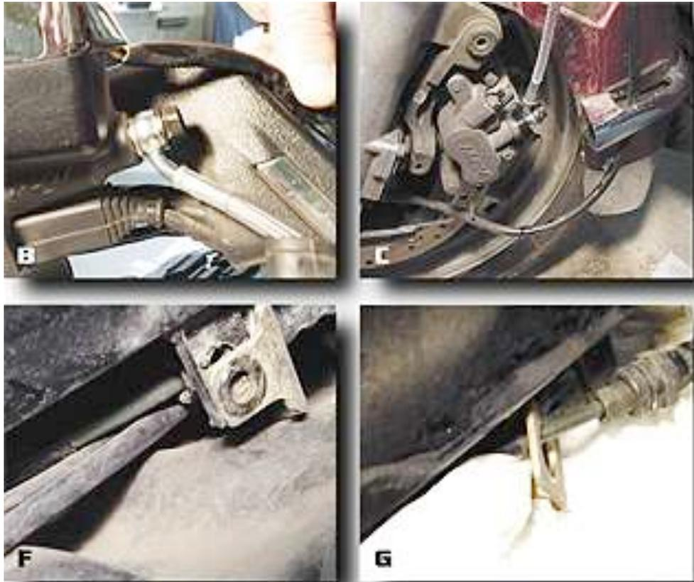
Next, using the new crush washers and the existing banjo bolt, connect the stainless steel line to the front caliper and tighten firmly. (Note both front calipers are connected in the same manner with the same hardware. (**Photo C.** is of left front caliper)
